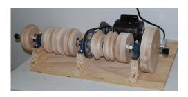
**Bob Brunson** has completed (except for the final arrangement of the wheels) his personal design of a sharpening station. With all these shapes he has run out of excuses for having dull, or even semisharp, tools.
